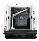
OPTION 3 - ESB - P30 Includes: 3-ft. fold-down crane, pedestal, reinforcement kit
